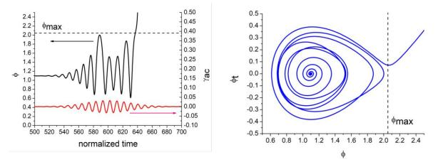
**Figure 6.** Simulation of the pulse induced switching. The single photon is simulated by a gaussian shaped oscillating current  $I_{ph}$ . The switching occurs when junction phase  $\phi$  crosses  $\phi_{max}$ . The horizontal axis is the normalized time, while the vertical axis is the junction phase (black curve) and the normalized current (red curve).
