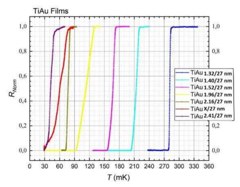
Figure 3. R vs T of various TiAu films, for different Ti/Au ratios (see legend), showing the possibility to engineer  $T_c$  and  $\alpha$ . The Ti thickness corresponding to the red curve is not reported because it is not regular.
