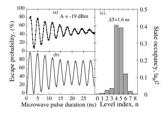
FIG. 3. (a) Measured escape probability versus MW pulse duration at the working point, defined by  $\Phi_{\rm dc}/\Phi_0=0.095$  and  $I_b=4.7~\mu{\rm A}$ , with about 15 levels localized in the anharmonic well. (b) Predicted escape probability for a MW amplitude  $\Phi_{\rm MW}/\Phi_0=0.002$ . (c)  $a_n$  coefficients of the state obtained after 1.6 ns duration of the MW pulse corresponding to the first maximum of the coherent oscillations.
