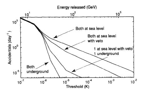
Figure 1. The number of accidental coincidences per day as a function of the detector burst threshold for different pairs of 40 ton aluminum spherical detectors.
