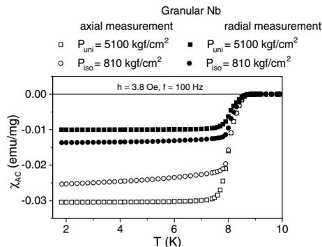
Fig. 2. AC-susceptibility of two Nb 3D-DJJAs, before and after application of an isostatic pressure, measured in both axial and radial geometries (see text).
