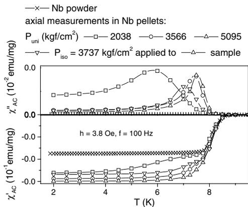
Fig. 1. AC-susceptibility of a Nb 3D-DJJA submitted to different pressures, measured in the axial geometry (see text).
