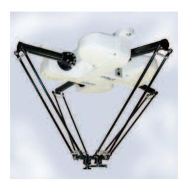
Figure 2.17: Adept Technology's Quattro robot, a parallel Schönflies–motion generator
