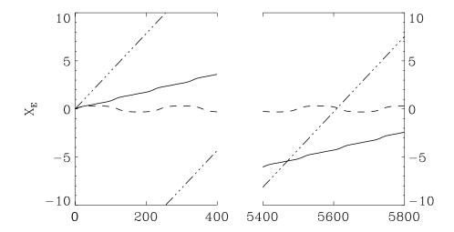
Fig. 3. Evolution of the center of energy (modulo 20) of a breather perturbed along its translation mode with various amplitudes:  $\lambda < \lambda_c$  (dashed line),  $\lambda \approx \lambda_c$  (full line) and  $\lambda > \lambda_c$  (dash-triple dotted line). The on-site potential is the Morse potential, C = 0.129 and the frequency of the breather is  $\omega_b = 0.80$ . The unit of time is the period of the perturbed breather.
