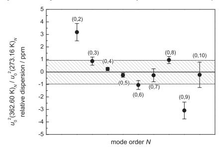
**Figure 14.** Relative differences between the squared speed of sound ratios  $[u_0^2(T)_N/u_0^2(T_{\text{TPW}})_N]$  of individual radial modes and the ratio  $\langle u_0^2(T)_N/u_0^2(T_{\text{TPW}})_N \rangle$  obtained by combining the weighted mean of four selected modes at two temperatures. The striped area and the solid lines display the uncertainty of the weighted mean estimate.
