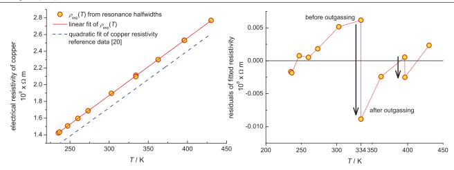
**Figure 4.** (Left panel) Comparison between the resistivity of copper, experimentally estimated from the resonance halfwidths and a literature estimate [22]. (Right panel) Residuals of a linear fit to our experimental estimated resistivity of copper. At 334 K and 396 K, glitches show the decrease of the resistivity presumably caused by outgassing absorbed impurities on the cavity surface.
