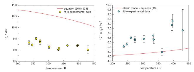
**Figure 11.** Comparison of the *breathing* frequency  $f_{br}(T)$  and the adiabatic compressibility of the shell  $\chi_S(T)$  as determined by reference models [36, 41] (red solid lines) or by fitting experimental acoustic data using equation (12). The error bars display the statistical uncertainty of the fitting procedure.
