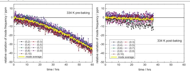
**Figure 16.** Relative variation of the resonance frequency of several acoustic modes recorded as a function of time at 170 kPa, 334 K before (left) and after (right) baking the cavity under vacuum at 450 K for one week. In both plots the records start at the instant t = 0 when the flow was stopped.
