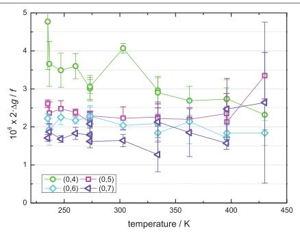
**Figure 8.** Excess halfwidths  $\Delta g = (g_{\text{exp}} - g_{\text{calc}})$  multiplied by the factor  $2 \times 10^6 / f_{\text{exp}}$  of four radial modes (0,4) to (0,7) as a function of temperature. Each plotted point and error bar represent the mean and the standard deviation of a set of data recorded along an isotherm at pressures between 170 kPa to 700 kPa.
