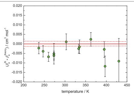
**Figure 12.** Comparison between the second acoustic virial coefficients  $\beta_a$  of He determined in this work (circles) and their accurate prediction from a recent first-principle [9] (red solid line). The error bars display the fitting uncertainty. The dashed lines delimit the uncertainty of the calculation.
