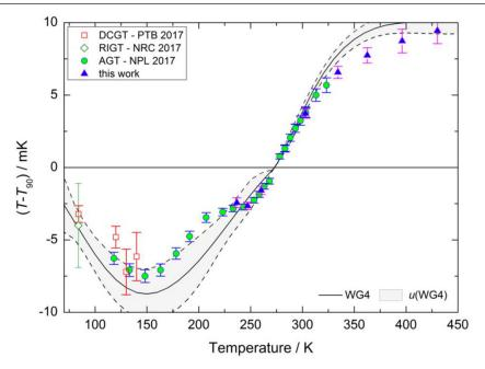
Figure 1. Differences between the thermodynamic temperatures obtained in this work and ITS-90.
