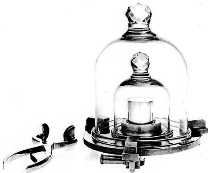
Figure 3.1. The Australian 1-kilogram standard, copy 44 of the BIPM 1 kilogram. The material is a platinum–iridium alloy and the cylinder has diameter equal to its height, each about 39 mm. The material is about 2.7 times denser than steel, implying a small volume for 1 kg and therefore a small buoyancy correction. The alloy has high resistance against corrosion and good electrical and thermal conductivities (Davis 2003).
