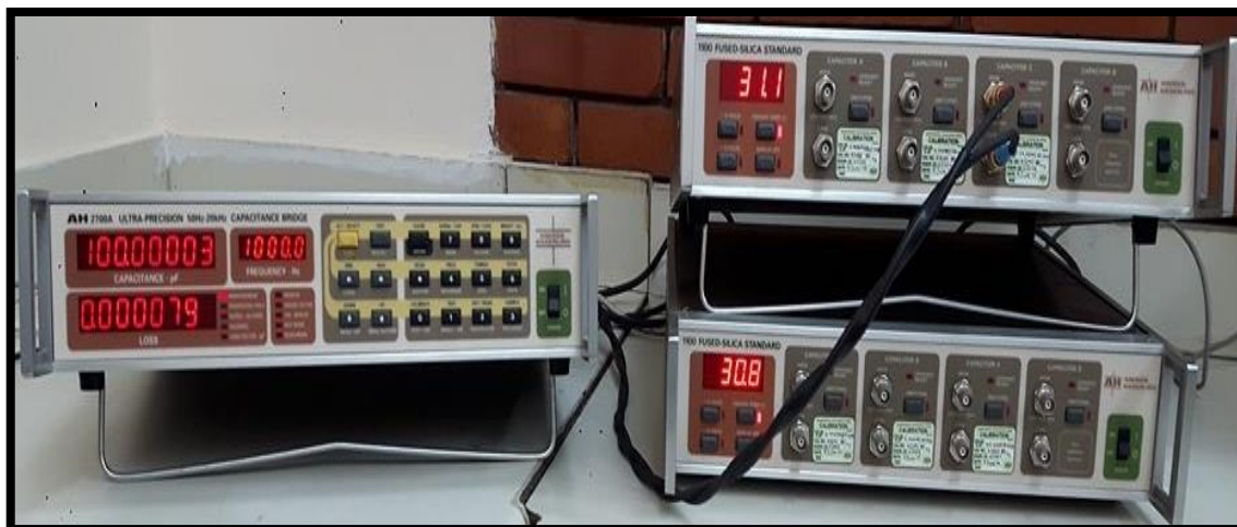
Figure 2. NIS capacitance measurement system formed by the latest AH bridge and the two highly accurate capacitance standards sets
