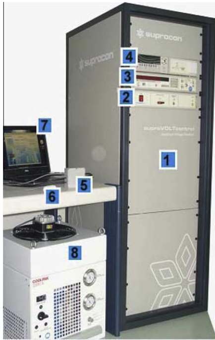
Fig. 49. The cryo-cooled Josephson voltage standard, fabricated ad Supracon AG. The system consists of the following components: 1: pulse tube cooler with a SIS Josephson junction array and the 75 GHz microwave electronics installed in the 19" rack, 2: control electronics, 3: source looking counter, 4: null detector, 5: 3-channel polarity reversal switch, 6: sensors for temperature, pressure and humidity, 7: computer control, 8: 2 kW compressor unit. Permissions received from M. Meyer, Supracon AG, Jena, Germany
