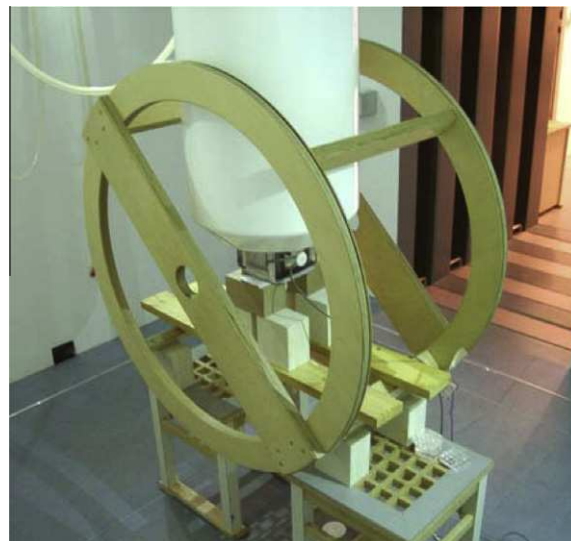
Fig. 27. Low-field NMR setup (PTB). The polarization field generated magnetization along the y-axis by the large Helmholtz coils. After switching off the polarization field, sample magnetization begins to precess about the z-axis of the detection field which is produced by a small field coil containing the sample below the cryostat. The LF-NMR setup is operated in a magnetically shielded room. Permissions received from L. Trahms, PTB Berlin, Germany
