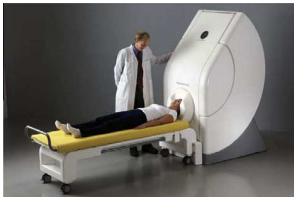
Fig. 26. Commercial LT SQUID MEG system providing sophisticated 3D mapping of brain activity. Source: Courtesy of [116]. Permissions received from L. Särnmann, Elektra Instrument AB, Stockholm, Sweden
