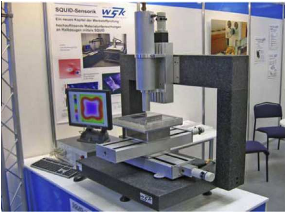
Fig. 29. Photography of commercial LT SQUID NDE system, Source: courtesy of [129]. Permissions received from M. Mück, ez SQUID, Sinn, Germany
