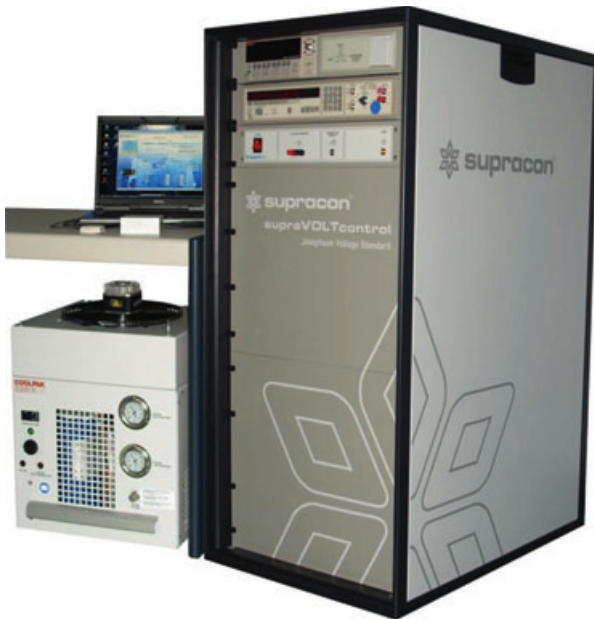
Figure 7.1.2 Photograph of a commercial cryocooler-based Josephson voltage standard system. (Courtesy of Supracon AG.)
