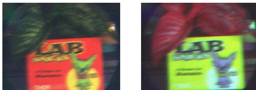
Figure 3. Example images acquired by the MAHI prototype operating in Color Imaging mode. Each image is assembled in software based on the acquisition of three single-band images, RGB (left) and Color Infrared (CIR) (right). The scene features a live plant with green leaves and white features and a brightly colored cardboard box. The addition of the infrared band in the CIR filter helps to discriminate live vegetation from inks with similar color. The programmable nature of MAHI's spectral filter enables customized band selection to highlight features of interest in any application and rapid switching between filters at video rates. (color in electronic version)
