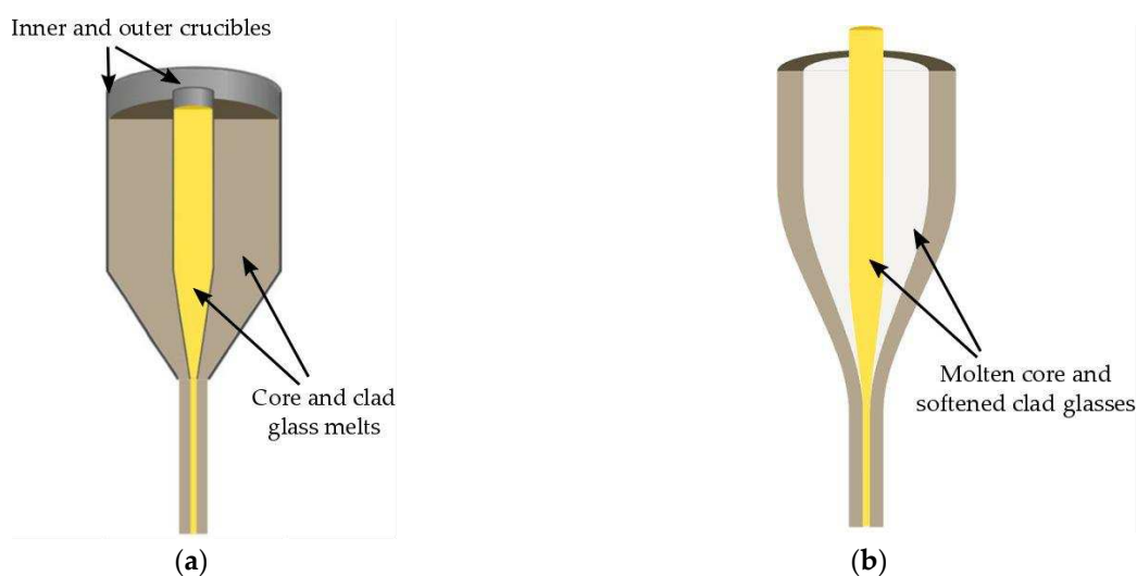
Figure 4. Principle (a) double-crucible techniques and (b) melt in tube techniques. Adapted with permission from [142], W. Blanc and B. Dussardier “Formation and applications of nanoparticles in silica optical fibers”, J. Opt. 2016 , 45 , 247–254. Copyright 2015 The Optical Society of India.
