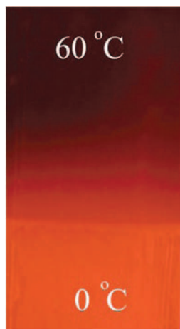
Fig. 24 Response of a planar T sensitive paint (film size 4 \times 7 cm). (Reprinted with permission from ref. 74. Copyright Wiley-VCH, 2006.) A heated planar sensor foil is dipped into ice water. The bright orange-red luminescence at 273 K (bottom) is less quenched compared to the less distinct luminescence at 333 K (top).
