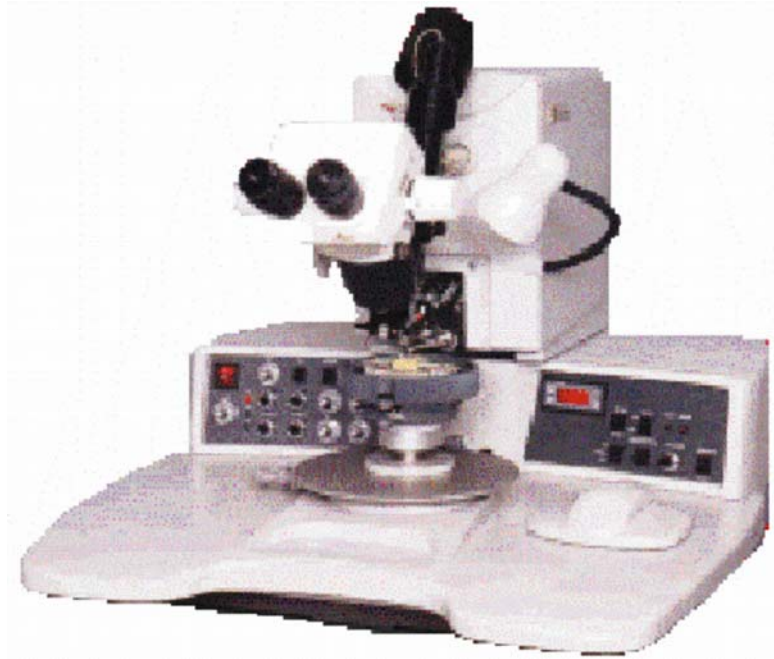
Figure 36) K&S 4124 Wire Bonder:
