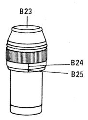
With knob (D 10) the brightness of these signs will be matched to that of the microscopic image. Without taking the microscopic image into consideration the eyelens mounts of the two WPK 10x eyepieces are rotated until in the left as well as in the right eyepiece the concentric circles are seen distinctly. Then the microscopic image is sharply focused with the fine control.
