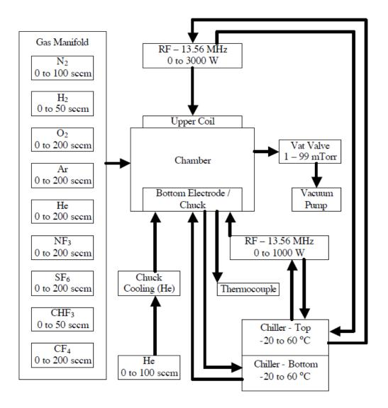
Block Diagram of Parameters Associated with the Chamber of the TCP 9400SE II system
