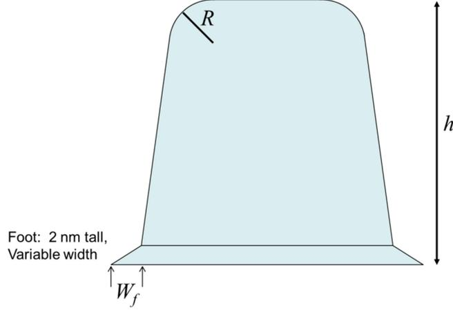
Figure 2. Geometry used to define the foot width  $W_f$  and top corner rounding radius  $R$ .
