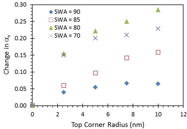
Figure 6. Fitting the ALM to Monte Carlo simulation results allows the step volume loss factor  $\alpha_v$  to be correlated with the top corner rounding radius. Here, the change in  $\alpha_v$ , compared to no top corner rounding is shown.
