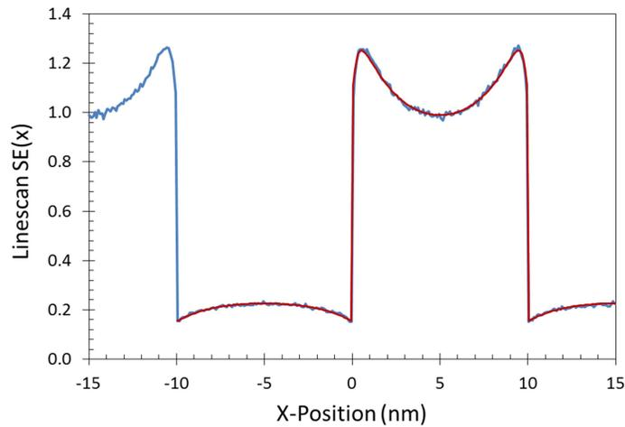
Figure 3. The ALM (red smooth curve) compared to the Monte Carlo simulation results (blue jagged curve) for 30-nm tall silicon features on a silicon wafer, SWA = 90°, 10-nm lines and spaces (RMS error = 0.0075).
