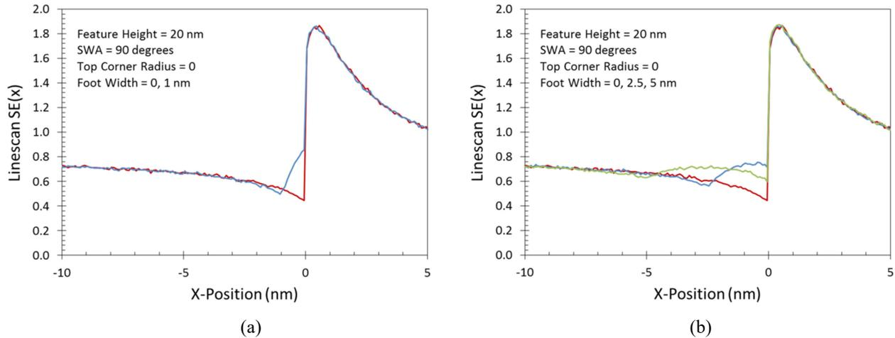
Figure 4. Monte Carlo simulation results showing the impact of a 2-nm tall trapezoidal foot of varying widths on the resulting linescan (20-nm tall, 90° silicon edge on a silicon wafer, 500 V, point beam of electrons). The linescans with and without a foot are compared for (a) a 1-nm wide foot, and (b) a 2.5-nm and 5-nm foot.
