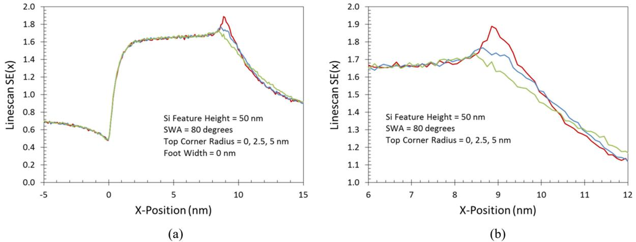
Figure 5. Monte Carlo simulation results showing the impact of top corner rounding of varying radii on the resulting linescan (50-nm tall, 80° silicon edge on a silicon wafer, 500 V, point beam of electrons). The linescans with and without corner are compared in (a) with the region around the peak magnified in (b).
