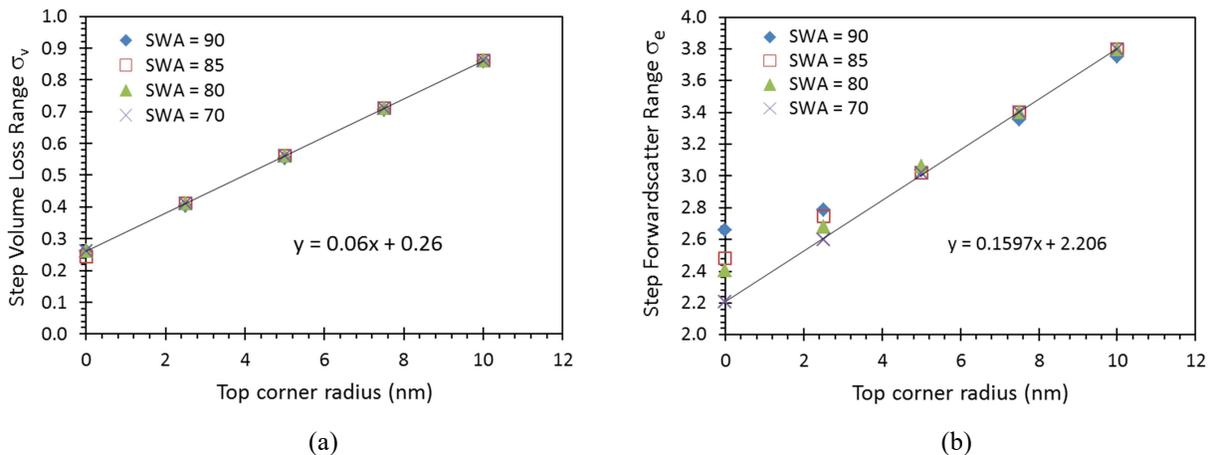
Figure 7. Monte Carlo simulation results showing the impact of top corner rounding of varying radii on two ALM parameters (20-nm tall silicon edge on a silicon wafer, 500 V, point beam of electrons): (a) the feature volume loss range  $\sigma_v$ , and (b) the feature forward scatter range  $\sigma_e$ .
