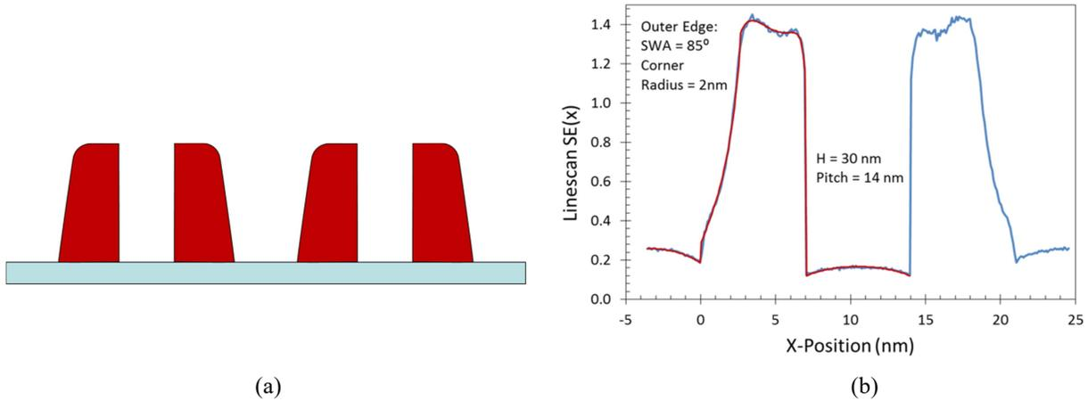
Figure 8. Applying the ALM to sidewall spacer features: (a) an example of a set of asymmetric sidewall spacer features, and (b) Monte Carlo simulated linescans (blue jagged line) with a best-fit ALM (smooth red line). The silicon feature lines and spaces were 7 nm wide at the bottom.
