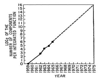
Fig. 1. Moore's 1965 prediction of the doubling of the number of "minimum cost" components on a chip each year, based on historical data and extrapolated to 1975 [4].
