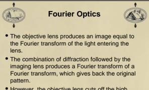
However, the objective lens cuts off the high spatial frequencies of the diffraction pattern.
