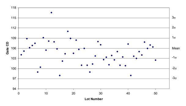
(b) For the data in part (a), the mean is 106 nm and the standard deviation is 3 nm. If the target CD is 105 nm and the specification limits are  $\pm 10\%$ , what is the Cpk of this process? Is this Cpk bad, marginal, good, or great?
