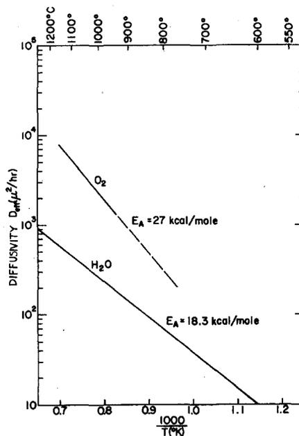
FIG. 10. The diffusivity of oxygen (Norton<sup>21</sup>) and of water (Moulson and Roberts<sup>22</sup>) in fused silica as a function of temperature.
