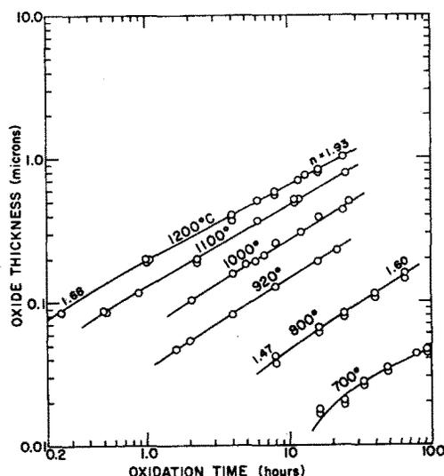
FIG. 2. Oxidation of silicon in dry oxygen (760 Torr).
