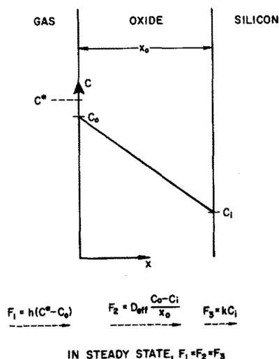
FIG. 3. Model for the oxidation of silicon.
