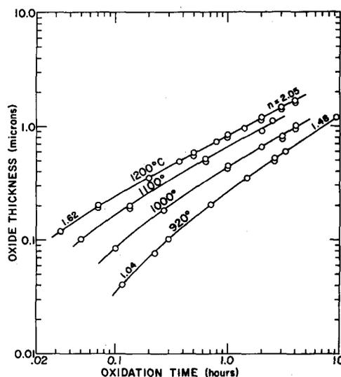
FIG. 1. Oxidation of silicon in wet oxygen (95°C H<sub>2</sub>O).
