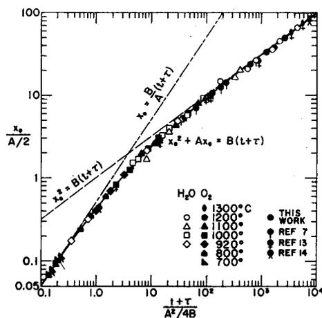
FIG. 12. General relationship for thermal oxidation of silicon. The solid line represents the general relationship, the dotted lines its two limiting forms. Experimental data were reduced using values of  $A$  and  $B$  determined from Figs. 8, 9, and 11. The values of  $\tau$  correspond to  $x_i = 0$  and  $200 \text{ \AA}$  for wet and dry oxygen, respectively.
