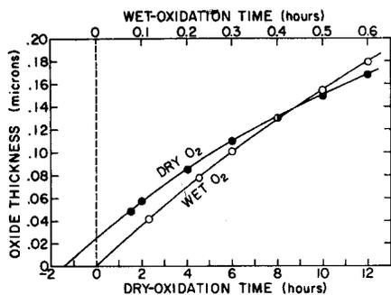
FIG. 5. Comparison of initial oxide growth at 920°C for oxidation in wet-(95°C H<sub>2</sub>O) and dry-oxygen ambients.
