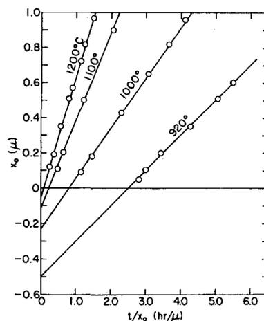
FIG. 4. Evaluation of rate constants for oxidation of silicon in wet oxygen (95°C H<sub>2</sub>O). Slopes of lines correspond to  $B$  in Eq. (12), intercepts at  $t/x_0=0$  correspond to  $-A$  in Eq. (12).
