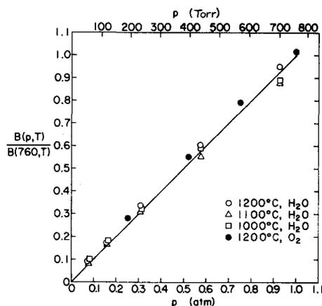
Fig. 8. The effect of partial pressure of the oxidant on the parabolic rate constant. Rate constants are normalized to the 760-Torr value at the same temperature. (Flint's<sup>7</sup> data for wet and dry oxygen, 1000° to 1200°C).
