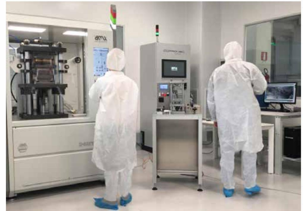
AMX Automatrix is able to sustain the customer during the process developing phase or for testing activities. ISO Class 6 clean room to simulate the entire sintering cycle.
