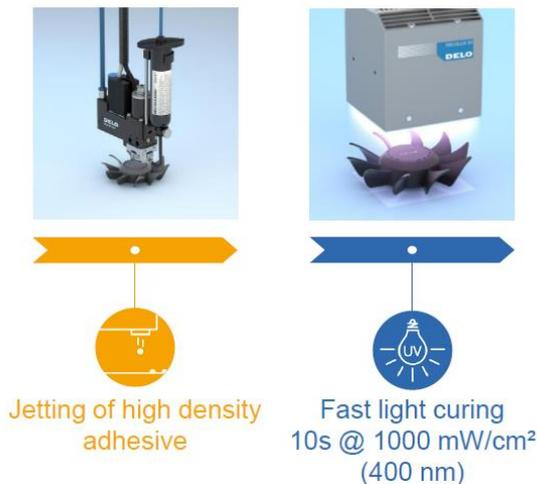
Figure 4 – A quantity of adhesive is applied to achieve balance and is then light cured. Image courtesy of DELO.
