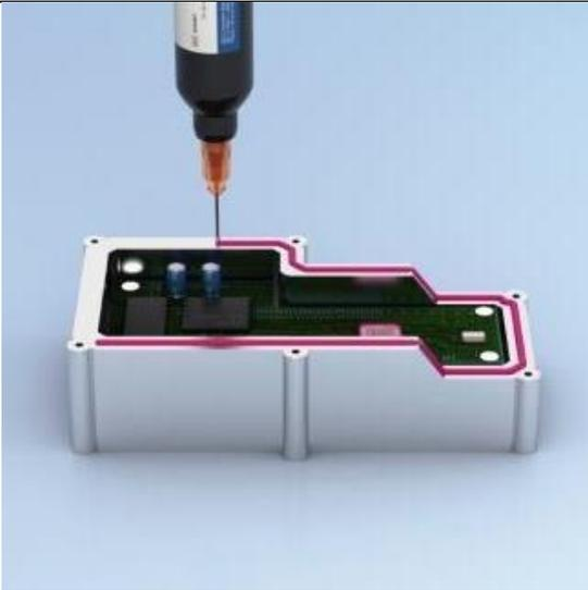
Figure 3 – One of the benefits of a CIPG is that complex-shaped gaskets can be easily created. Image courtesy of DELO.
