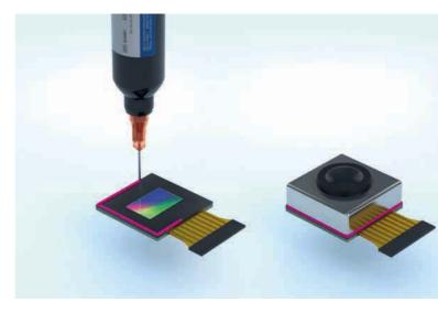
However, if too much energy is provided, there will not be enough time to place the second substrate in position before a skin forms on the surface of the adhesive. Once this happens, it is impossible to bond the substrates.
