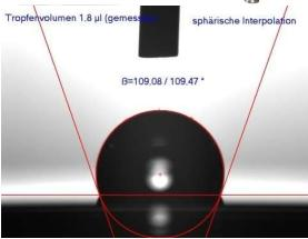
A small investment of time used to measure the contact angle can give a large return by avoiding later production problems. To reduce defect density and feature sizes of resist
