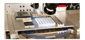
Many different holders for various substrate and package types, waffle/gel packs (2", 4") and trays
