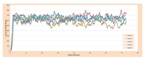
Force per unit width vs. Distance peeled for five samples of an adhesive tape of the same batch
