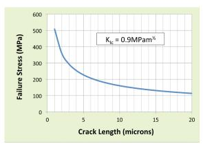
Impact of crack length on failure stress for silicon
