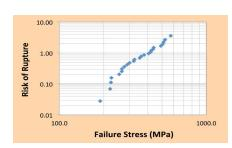
Weibull distribution of failure stress from 3pt micro bend measurements
