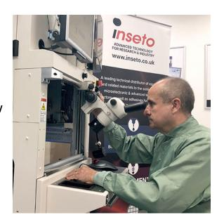
Andover, United Kingdom – Inseto, a leading technical distributor of equipment and materials, has invested in a Kulicke & Soffa (K&S) Asterion wedge bonder. Located in Inseto's new Process Development Laboratory along with materials test and plasma cleaning equipment, the automatic bonder is suitable for the large-wire, fine-wire and ribbon bonding of hybrid circuits, semiconductor devices, sensors, and automotive power modules and battery packs.
