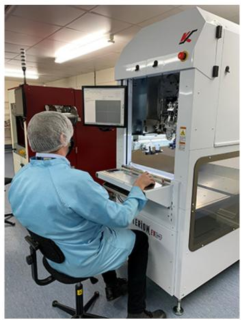
Supplied by Inseto, CIL's new Kulicke & Soffa Asterion large diameter wire / ribbon wedge bonder will be used for the production of wide bandgap (WBG) semiconductor-based power modules and the assembly of battery packs for use in electric vehicles.
