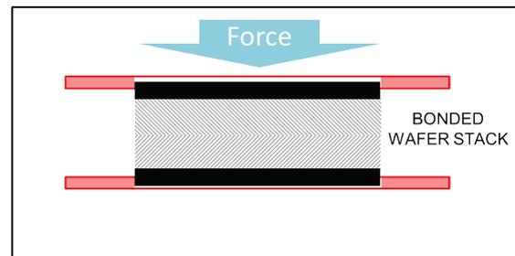
5) Apply force to bring wafers into contact & bond
