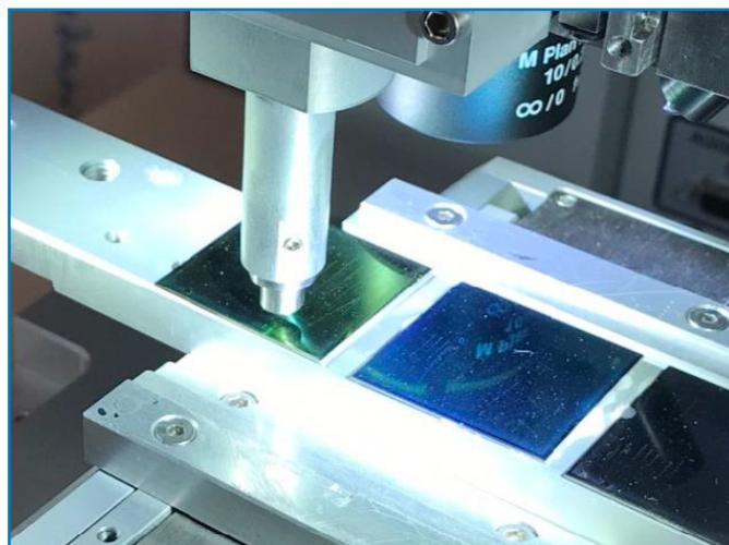
**Figure 4.** Scratch testing set-up on a ceramic coating.
