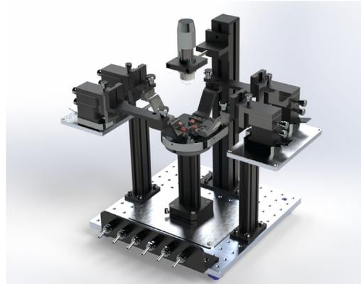
The SemiProbe Mini-PS4L family of probe systems are built using the same design concepts as our patented Probe System for Life (PS4L) Architecture. The Mini-Series is designed to address the requirements of small sample testing using a small footprint.
