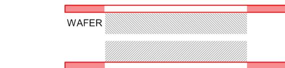
3) Load second wafer and align if required
