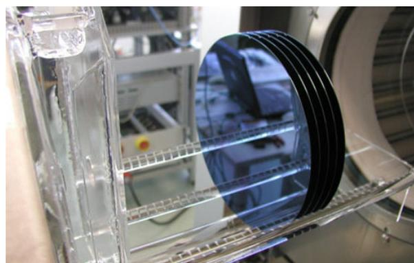
200mm Horizontal oxidation furnace, (image courtesy of [ATV](#))
