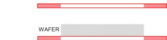
2) Load first wafer to be bonded
