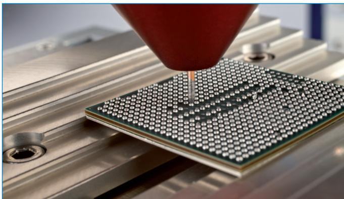
Close up of copper probe on BGA
