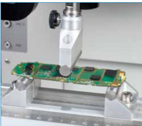
Bend testing of final assembly
