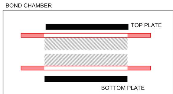
4) Load transport fixture and wafers into bond chamber
