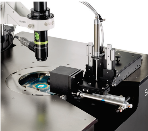
Semi-automatic equipment for 150mm wafer probe testing optoelectronic devices
