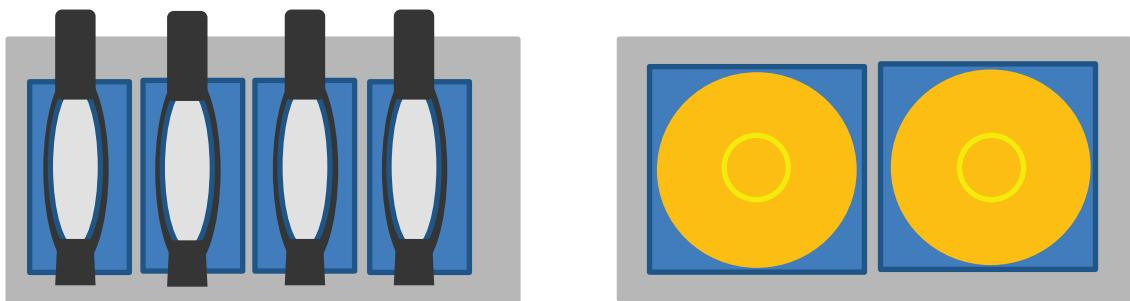
Wedge Bond versus Ball Bond Pitch Comparison
