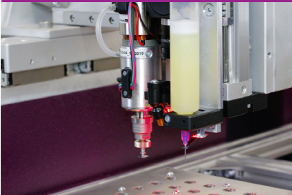
Free moveable writing time/pressure or rotary micro valve dispenser
