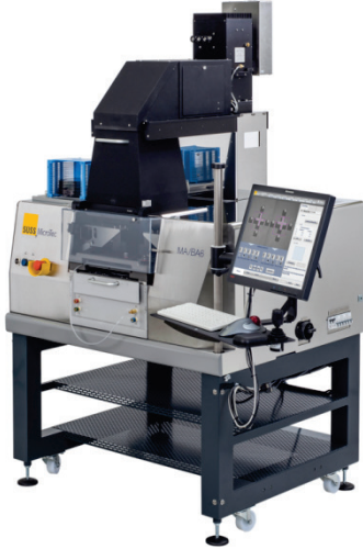
SUSS Mask Aligner with LED Light Source
