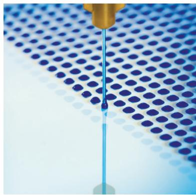
This will be heavily influenced by the joining agent, and the substrates being joined. Solder preforms (and cut ribbon) are either placed by hand (R&D, prototyping) or by die bonders, also known as pick-and-place machines, for high volume production. The cost of die bonders is dictated by the required UPH and repeatable placement accuracy. Solder paste is either dispensed or screen / stencil printed, depending on the size and topography of the substrate.
