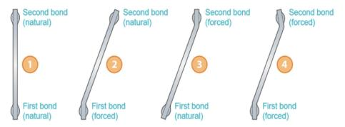
Note: Natural or forced angle diagram above shows a two dimensional bond head movement; actual movement occurs in three dimensions with rotation.
