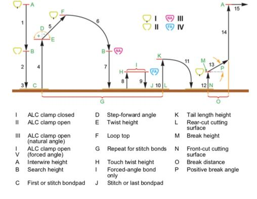
Note: Above shows a two dimensional bond head movement, Actual movement occurs in three dimensions with rotation.
