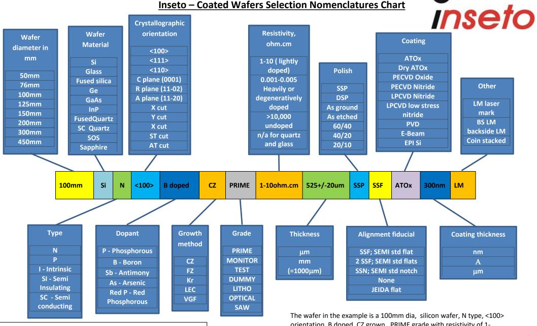
Inseto (UK) Limited Unit 25 Focus Way Andover, SP10 5NY United Kingdom +44 (0)1264 334505 - enguiries@inseto.co.uk - www.inseto.co.uk orientation, B doped, CZ grown, PRIME grade with resistivity of 1-10ohm.cm, thickness is 525+/-20um and it is single side polished with SEMI std flat.
