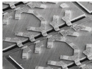
True-chip-size packages of HF devices
