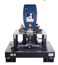
Systems integrated with the powerful Polytec MSA-500 laser Doppler Vibrometer system enable users to accurately measure the motion in actuators, energy harvesting or any other device with moving parts.
