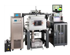
Vacuum probers are used for resonators, sensors and any other MEMS product that will eventually be packaged in a vacuum. Wafer level test saves money by providing known good die (KGD) before expensive packaging as well as determining the optimal vacuum level for the package.
