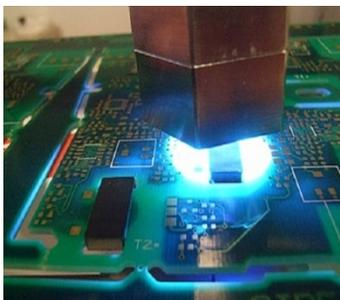
For applications where cycle time does not allow for lengthy heat cure stages (even when carried out off-line), or where one of the materials being bonded is sensitive to temperatures even as low as 80°C (as a lot of new, low-cost plastics tend to be), then serious consideration needs to be given to light-activated adhesives.
