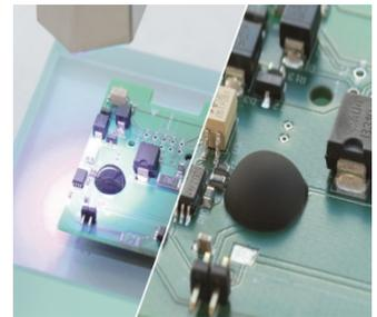
Regardless of where on the spectrum the Photoinitiator lies, the simple fact is that one of the parts being bonded must be transparent, to allow for 100% cure of the adhesive. No one likes having uncured adhesive in their products on a long-term basis, especially as a number of these adhesives are based on acrylic acid (rendered harmless by curing).
