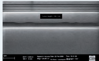
UV-NIL: 50nm, 70nm lines and spaces imprinted with MJB4 Mask Aligner
