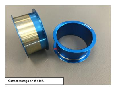
Bonding wire is usually spooled from one end of a spool to the other in a single layer. Each end is usually secured to the edge of the spool with a piece of coloured tape. Each end of the wire will have a different colour indicating the start and the end of the spool. It is important when starting a new spool to check the manufacturer's instructions on what end is the beginning, this information will usually be on the packaging of the wire spools.
