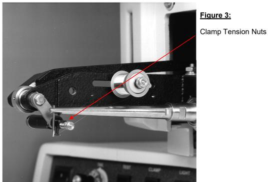
Repeat steps 1 - 4, however, turn the nuts clockwise (towards the solenoid) until the wire breaks cleanly.
