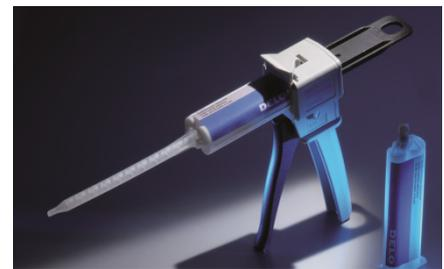
**Acrylates.** Predominantly transparent, these are one-part adhesives and are cured using heat and/or light, have a shelf-life of between six months and a year and, once cured, exposed surfaces remain tacky. At about 30MPa, acrylates are more flexible than epoxies. Storage requirements will vary from 0°C to room temperature.
