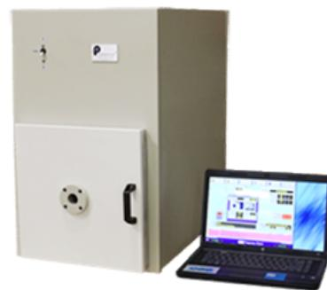
Low Pressure Plasma Cleaning involves the removal of impurities and contaminants from surfaces through the use of energised plasma created from gaseous species. Gases such as Argon and Oxygen are used, as well as mixtures such as air and Hydrogen / Nitrogen. The plasma is created by using high frequency (RF) voltages (typically >10MHz) or Microwave frequency voltages to ionize the low-pressure gas (typically around 150mTorr-400mTorr), although atmospheric pressure plasmas are now also common.
