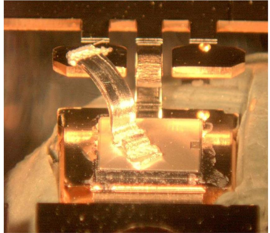
Note: Single Bond And Change In Elevation With Low Loop Characteristics
