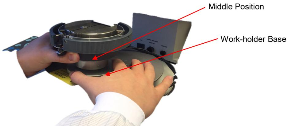
6. Rotate workholder anticlockwise fully to lowest position.
