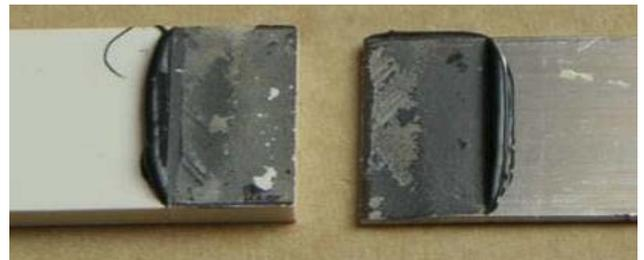
Flexibility – there are different ways to indicate the flexibility of an adhesive: elongation, Young’s Modulus, sometimes shore hardness. Elongation is the easiest to both measure and visualise – it is calculated in the same test that determines the tensile strength of the adhesive. The percentage that the test coupon has strength when it breaks is the elongation, also specified in the data sheet – simple!
