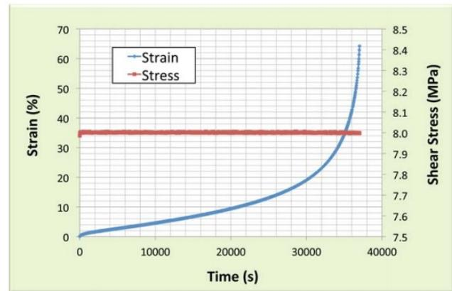
The left image shows creep testing on solder balls, the right image shows creep data for a 60/40 SnPb solder.
