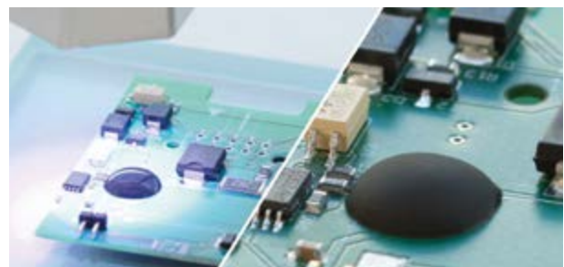
Defined glop top encapsulation within seconds (left during curing, right after curing)
