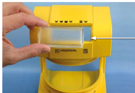
Bonding a display plate made of PC into a powder-coated aluminum housing
