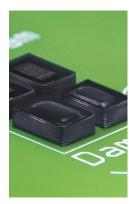
Thanks to a very high viscosity of 160,000mPas, the adhesive also provides high flow resistance and an aspect ratio of 2.5. This means that the height of an adhesive bead can be more than twice its width, without the bead collapsing. In addition DELO MONOPOX GE7985 has low water absorption and a very good resistance to acids, oils and other aggressive media.
