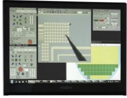
PILOT software suite main screen display with Navigator and Wafer Map Modules, microscope and manipulator controls and integrated video display
