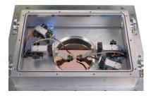
Platen surface shown with programmable manipulators for high frequency and DC testing
