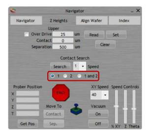
**Navigator Z Set-Up** – user has the flexibility of setting the contact, separation and overdrive. Automatic contact search and speed is user selectable.
