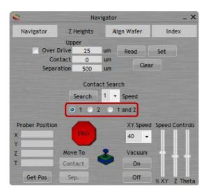
**Navigator Z Set-Up** – user has the flexibility of setting the contact, separation and overdrive. Automatic contact search and speed is user selectable.
