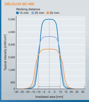
Light intensity distribution in dependence of the distance between lamp head and bonding area
